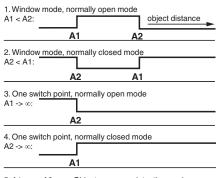
5. A1 ->  $\infty$ , A2 ->  $\infty$ : Object presence detection mode Object detected: Switch output closed No object detected: Switch output open
