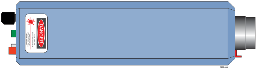
Figure 7. Top view of laser showing the location of the “Warning logotype” label for a Class IIIa laser.
