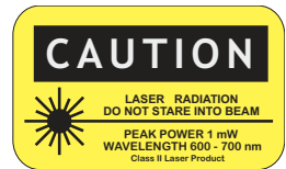
Figure 4. Warning logotype label for Class II lasers.
