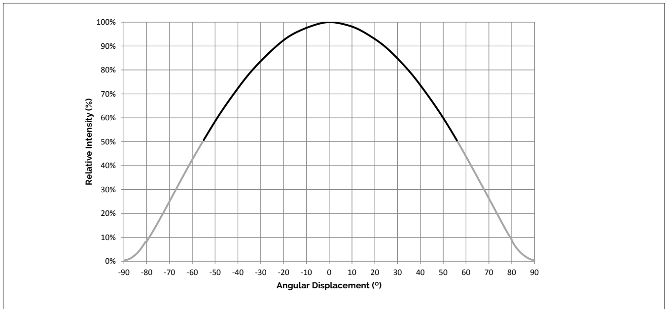
Figure 10: Typical Spatial Radiation Pattern
