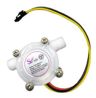
Water flow sensor consists of a plastic valve body, a water rotor, and a hall-effect sensor. When water flows through the rotor, rotor rolls. Its speed changes with different rate of flow. The hall-effect sensor outputs the corresponding pulse Signal.
