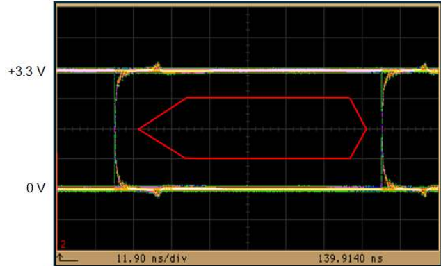
Figure 11. USB 1.1 Full Speed Eye Diagram
