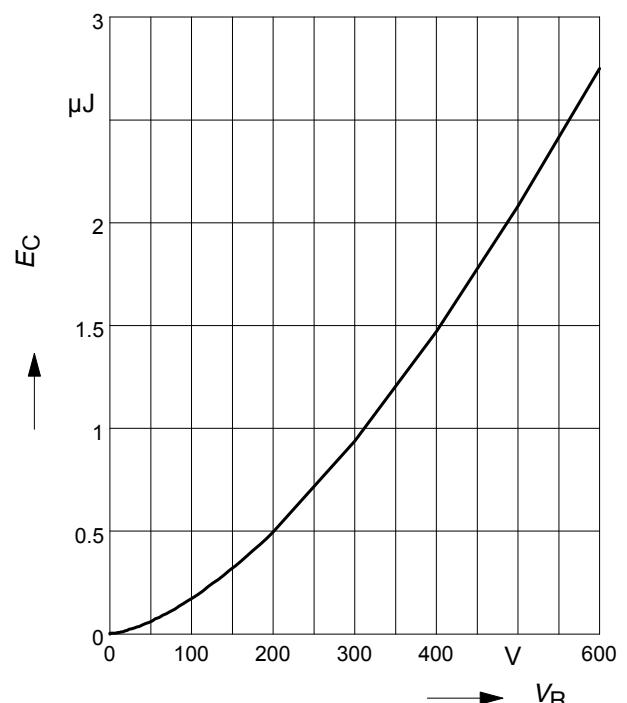
**9 Typ. capacitive charge vs. current slope**
