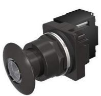
30mm BlackMax, Epoxy Coated Corrosion Resistant Complete Metal Unit Illuminated Push-Pull Operator Full Voltage, 12V AC/DC Incandescent Lamp Mushroom Head Cap Small 1 3/4" (44.5 mm) Metal, Black with Clear Lens 3 Position Pull-Momentary/Push-Maintained UL Listed, CSA Certified NEMA 1,3,3R,4,4X,12,13 & Automotive Standards
