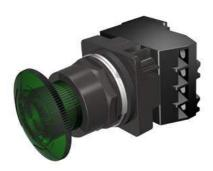
30mm BlackMax, Epoxy Coated Corrosion Resistant Complete Metal Unit Illuminated Twist-to-Release Transformer type, 600V AC Incandescent Lamp Mushroom Head Cap Small 1.79" (45 mm) Plastic Cap, Green 2 Position Maintained, Twist-to-Release with 1 N.O. - 1 N.C. Heavy Duty Contacts, A600/P600 UL Listed, CSA Certified NEMA 1,3,3R,4,4X,12,13 & Automotive Standards
