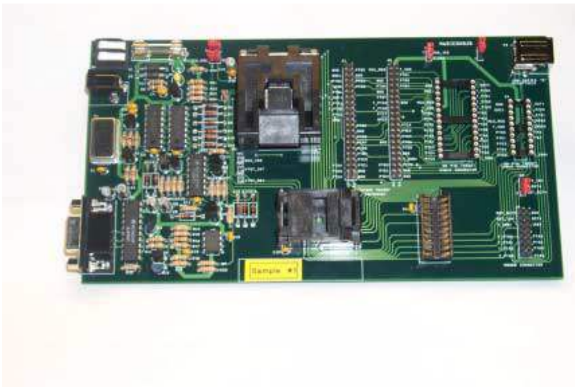
Figure 1-1 M68ICS08JB In-Circuit Simulator Board
