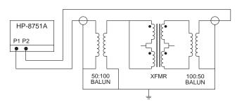
4. Crosstalk Attenuation — In the dual packages, which contain transmit and receive transformers side by side, sufficient crosstalk attenuation is achieved by the inherent characteristics of the toroid cores as well as by their proper positioning. The crosstalk attenuation is typically 50 dB or better from 100 kHz to 10 MHz. This result was established with the test circuit shown below.
