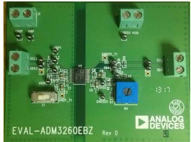
Figure 1. EVAL-ADM3260EBZ Evaluation Board
