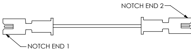
-NUS (END 2 NOTCH UP, CABLE STRAIGHT) (PIN 1 TO PIN 1)
