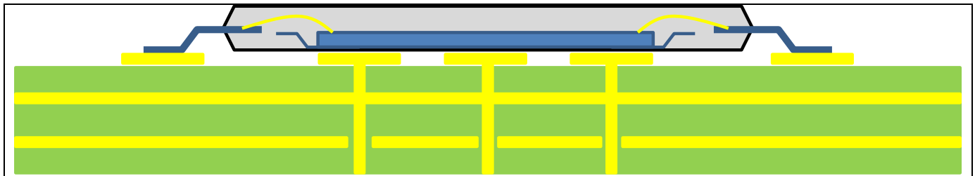
Figure 8-1: Example Thermal Via Holes on PCB
