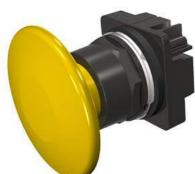
30mm BlackMax, Epoxy Coated Corrosion Resistant Metal Operator, Round Push-Pull Operator Non-Illuminated Mushroom Head Cap Large 2 1/2" (63.5 mm) Plastic, Yellow 3 Position Pull-Momentary/Push-Maintained UL Listed, CSA Certified NEMA 1,3,3R,4,4X,12,13 & Automotive Standards
