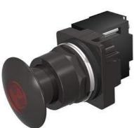
30mm BlackMax, Epoxy Coated Corrosion Resistant Complete Metal Unit Illuminated Push-Pull Operator Full Voltage, 120V AC/DC Incandescent Lamp Mushroom Head Cap Small 1 3/4" (44.5 mm) Metal, Black with Red Lens 3 Position Pull-Momentary/Push-Maintained UL Listed, CSA Certified NEMA 1,3,3R,4,4X,12,13 & Automotive Standards
