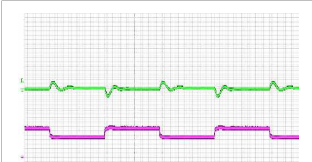
Output voltage response to load current step- change (0.42-0.63-0.42 A) at: T_{P1} = +25^{\circ}\text{C} , V_i = 48\text{ V} . Top trace: output voltage (2 V/div.), Bottom trace: load current (500 mA/div.), Time scale: (500 \mu\text{s} /div.).
