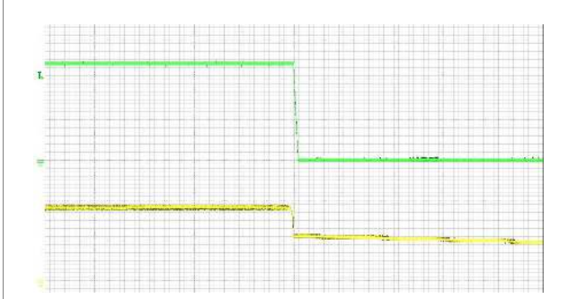
Start-up enabled by connecting V_i at: T_{P1} = +25^{\circ}\text{C} , V_i = 9\text{ V} , I_o = 1.67\text{ A} resistive load. Top trace: output voltage (10 V/div.), Bottom trace: input voltage (5 V/div.). Time scale: (20 ms/div.).
