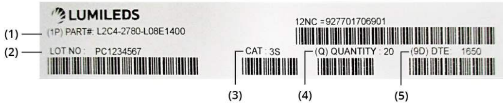
Figure 10. Example of a tube label for LUXEON CX Plus CoB.
