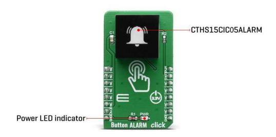
The alarm symbol icon on the top of the touch sensor is visible even when the backlight is off, thanks to the LEXAN™ polycarbonate film with an inverse print of the icon, placed on a top of the sensor. When the internal LEDs are turned ON, the light will pass through the translucent power symbol icon, resulting in a uniformly lit power symbol icon. An interesting lighting effect can be designed when touched, by applying a PWM signal to the IN pin.
