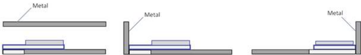
Fig 5-4. Not recommended location in Z plane
