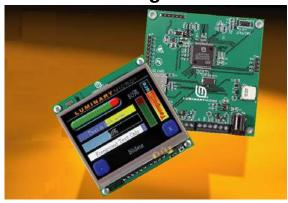
In addition to being offered as a stand-alone, ready-for-production module (MDL-IDM-L35), the Stellaris® IDM-L35 is also offered as a complete open-tool reference design kit (RDK-IDM-L35). The RDK ships with everything needed to quickly evaluate the IDM-L35 including:
