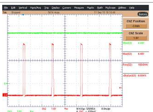
Figure 8-9. Supply Voltage 5 V Peak Signal 4.5 V
