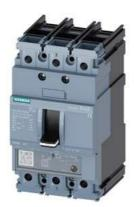
circuit breaker 3VA5 UL frame 125 breaking capacity class M 35kA @ 480 V 3-pole, line protection TM230, FTAM, In=60A overload protection Ir=60A fixed short-circuit protection Ii=5...10 x In UL489 SB (naval), 50 deg. cel. cable connection on both sides
