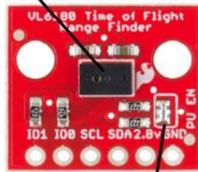
VL6180 Breakout Diagram
