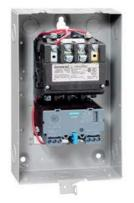
Non-reversing motor starter Size 1 Three phase full voltage Solid-state overload relay OLRelay amp range 10-40a 240VAC 50HZ / 277VAC 60HZ coil Combination type Indoor general purpose use
