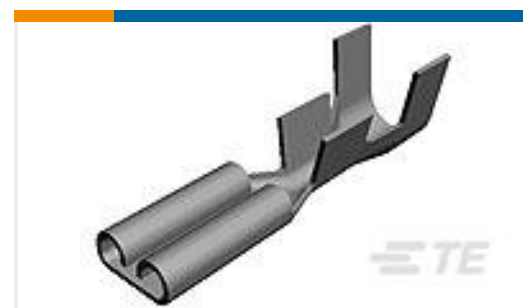
TE Part #63445-4 250 FASTON FLAG REC 18-12 AWG TPBR
