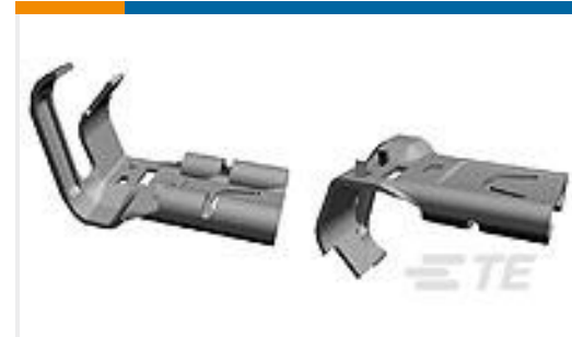
TE Part #63445-4 250 FASTON FLAG REC 18-12 AWG TPBR
