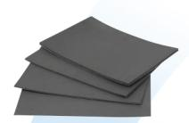
Q-ZORB PN 2238, RFSW-S-040-FR is a flexible elastomeric magnetic absorbing material. The material is designed to perform well for surface current attenuation. It can be used to lower the Q of cavities and reduce EMI. It is easily bonded using contact adhesives or it can be supplied with a pressure sensitive acrylic adhesive (PSA).
