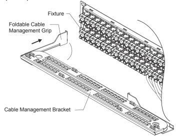
5. Fix the solid cables to the cable fixture hole using cable ties.
