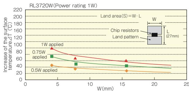
These high-power low resistance chip resistors are designed to dissipate heat efficiently through the land patterns on circuit boards. The actual temperature of the surface of the resistor is dependent upon the dimensions and the shape of the land patterns.
