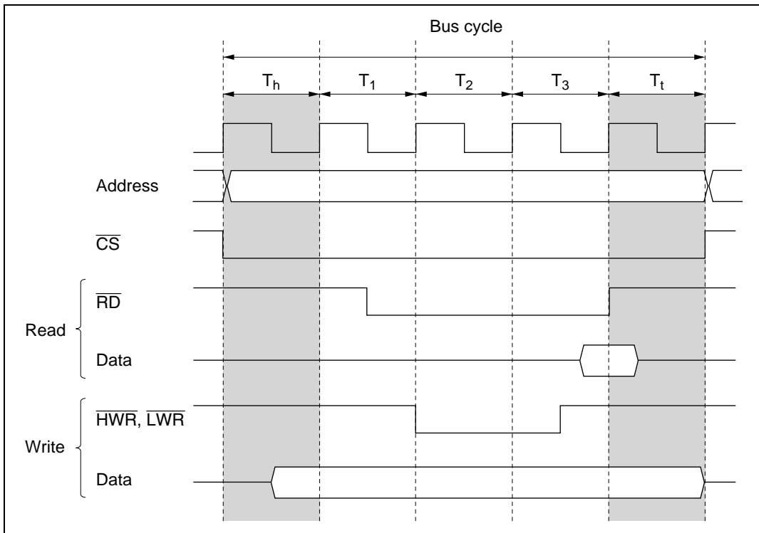
Figure 6.3 \overline{CS} and Address Assertion Period Extension (Example of 3-State Access Space and RDNn = 0 )
