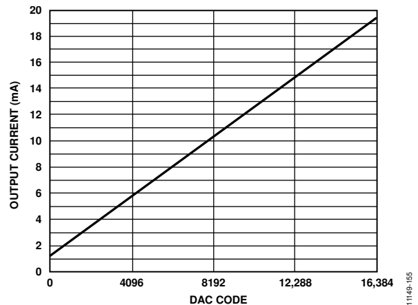
Figure 151. Gain Curve for FSC_x[9:0] = 512, DAC Offset = 1.228 mA
