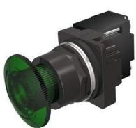
30mm BlackMax, Epoxy Coated Corrosion Resistant Metal Operator, Round Illuminated Twist-to-Release Transformer type, 120V AC LED Lamp Mushroom Head Cap Small 1.79" (45 mm) Plastic Cap, Green 2 Position Maintained, Twist-to-Release UL Listed, CSA Certified NEMA 1,3,3R,4,4X,12,13 & Automotive Standards
