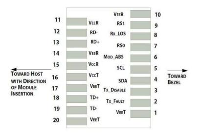
Pin-out of connector Block on Host board
