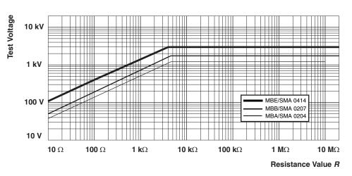
Pulse load rating in accordance with IEC 60115-1, 4.27; 10  $\mu$ s/700  $\mu$ s; 10 pulses at 1 minute intervals; for permissible resistance change (0.5 % R + 0.05  $\Omega$ ) **10/700 Pulse**
