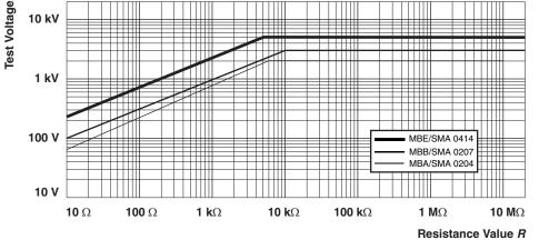
Pulse load rating in accordance with IEC 60115-1, 4.27; 1.2  $\mu$ s/50  $\mu$ s; 5 pulses at 12 s intervals; for permissible resistance change (0.5 % R + 0.05  $\Omega$ )
