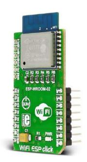
**WiFi ESP click** carries the ESP-WROOM-02 module that integrates ESP8266EX. The click is designed to run on a 3.3V power supply. It communicates with the target microcontroller over UART interface and the following pins on the mikroBUS<sup>TM</sup> line: RST, CS.
