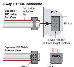
The **CAB-ISP6W200** is a **6-way** In-System Programming (ISP) ribbon cable designed to connect from any ISP programmer which features a 6-way IDC connector to a 6-way 0.1" pitch IDC connector on a suitable Target System. The cable features 200mm of flat ribbon cable with a 6-way IDC 0.1" pitch female connector on each end. The IDC connectors are fitted with 'cable grips' and are bump polarised to prevent the connector being plugged in the wrong way around.
