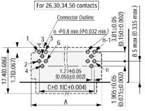
▼ =Polarity identification Recommended PCB Thickness t=1.6±0.19(0.063±0.007) "n" is number of contacts.
