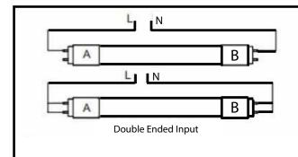
Input voltage: 120-277Vac 50/60Hz
