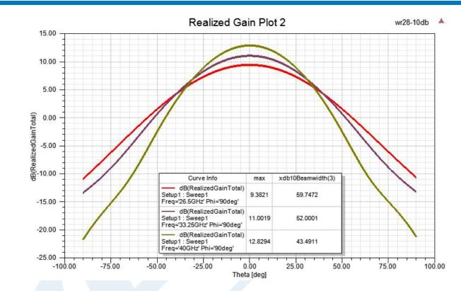
WR-28 Standard Gain Horn with 10 dBi gain, 2.92mm Female connector from Pasternack Enterprises has same day shipment for domestic and International orders. Our RF, microwave and millimeter wave products maintain a 99.4% availability and are part of the broadest selection in the industry.
