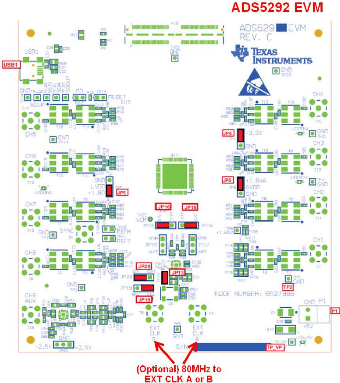
Figure 2. ADS5292EVM Basic Configuration
