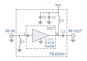
Fig 1. Application and Characterization Circuit
