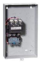
Non-reversing motor starter Size 3 1/2 Three phase full voltage Solid-state overload relay OLRelay amp range 50-200A 208VAC 60HZ coil Combination type Indoor general purpose use
