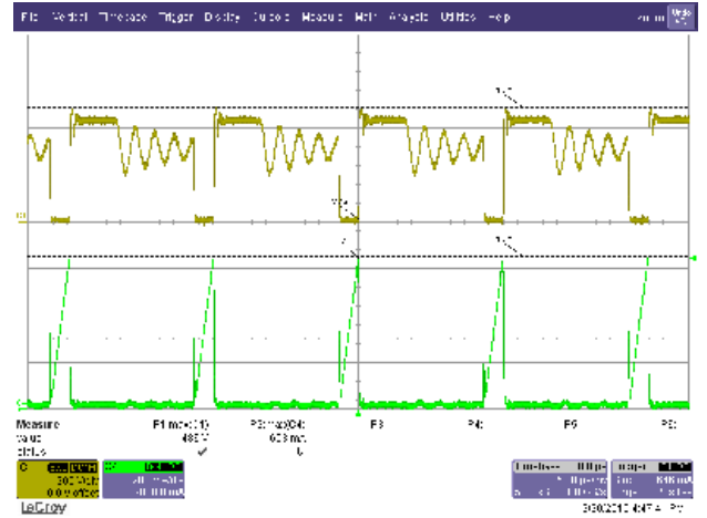
Figure 30 – 230 VAC / 50 Hz, 6 LED in Series (18.2 V / 350 mA). Upper: V_{DRAIN} , 200 V / div., 5 μs / div. Lower: I_{DRAIN} , 0.2 A / div.
