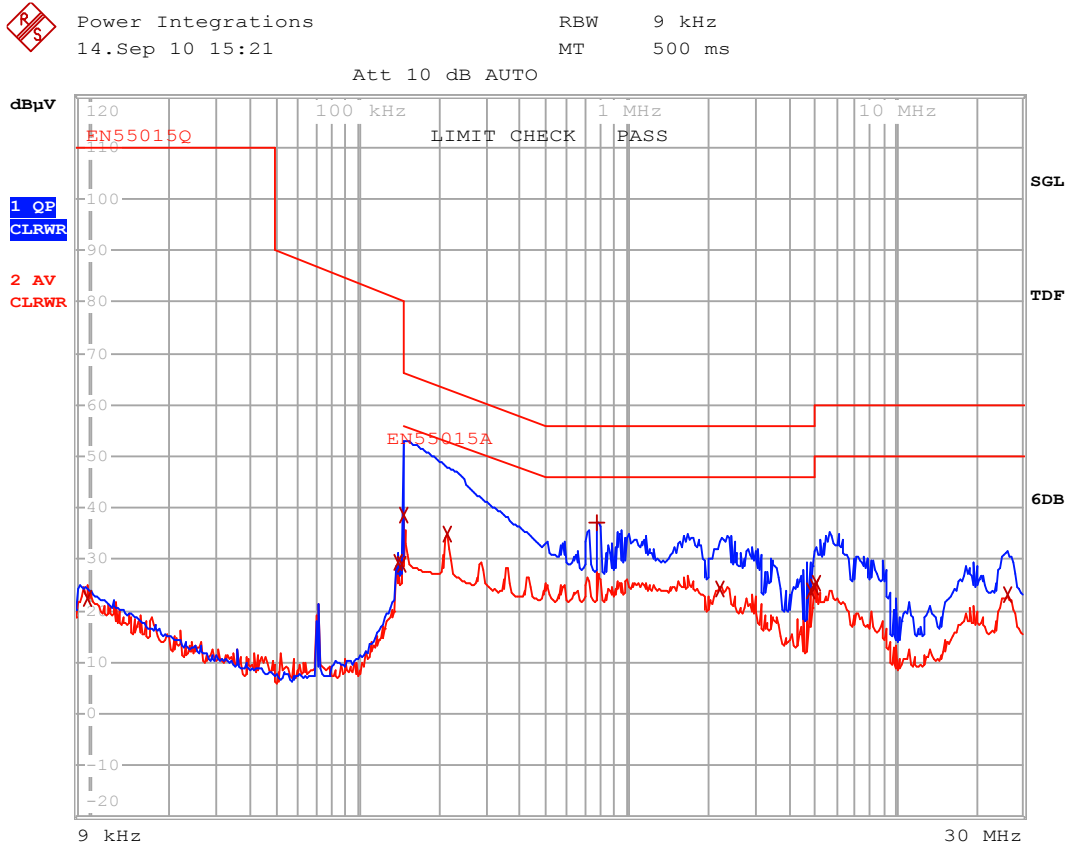
Figure 81 – Pre-scan Conducted EMI, Maximum Steady State Load, 230 VAC, 60 Hz, and EN55015 Limits. Note Blue Line is Peak Result vs. QP Limit Line – Refer to Table for QP Margin.
