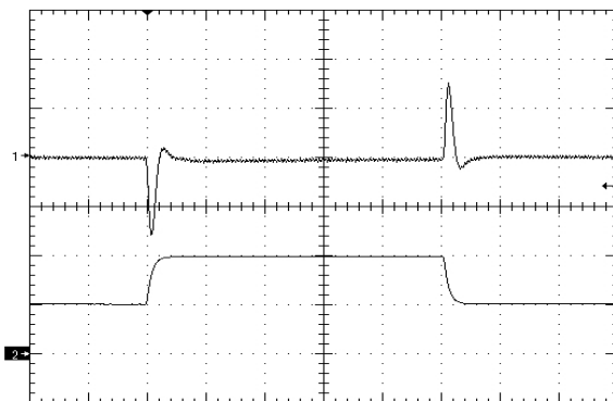
Figure 10. Load Transient Response (100mV/div), di/dt=0.1A/uS, 50% - 75% - 50% of full load, time scale: 200uS/div.
