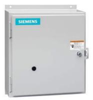
Mechanically held lighting contactor, Contactor amp rating 60Amp 0NC \_ 8NO poles, 24VAC 60HZ coil, Non-combination type, Enclosure NEMA type 1, Indoor general purpose use
