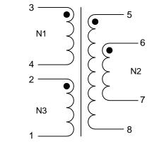
N2 denotes two windings connected in parallel. Terminals 5+6 and 7+8 must be tied as solder bridging is allowed.
