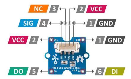
1 : Connected to the system GND
