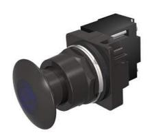
30mm BlackMax, Epoxy Coated Corrosion Resistant Complete Metal Unit Illuminated Push-Pull Operator Transformer type, 120V AC Incandescent Lamp Mushroom Head Cap Small 1 3/4" (44.5 mm) Metal, Black with Blue Lens 3 Position Pull-Momentary/Push-Maintained UL Listed, CSA Certified NEMA 1,3,3R,4,4X,12,13 & Automotive Standards
