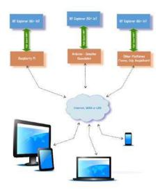
Furthermore, other platforms such as BeagleBone, Chip, Chipkit, Teensy all them can easily control a RF Explorer 3G+ IoT by manually connecting to a standard UART port.
