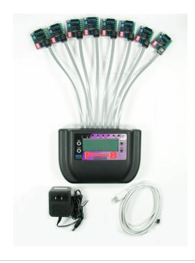
The Prime8 production programmer has eight high-speed ISCP $^{\text{TM}}$  jacks for high volume programming. Ideal for production environments, it can operate as a stand-alone production programmer with its SD card reader, or with CCS software on the PC. Program up to 8 devices individually or concurrently.
