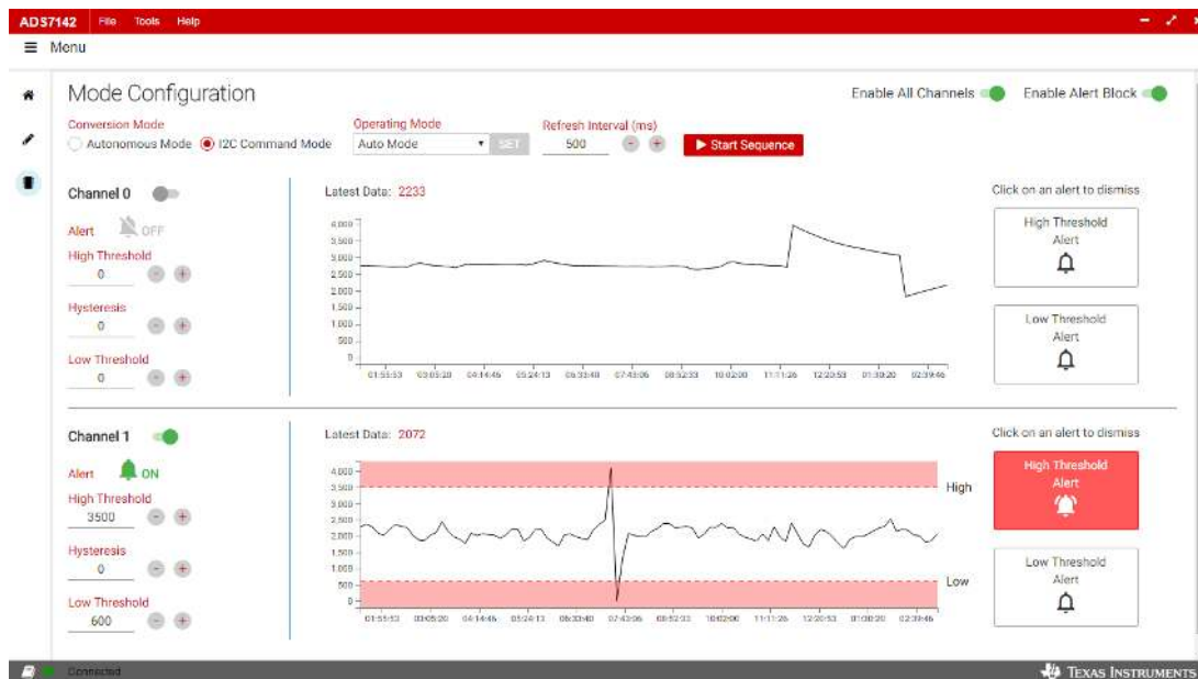
Figure 121. Alert Output from ADS7142 with PIR Sensor
